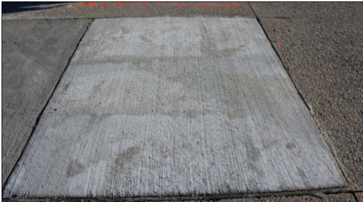
Figure 5.9: Staining mark on Panel 1A after burlap removal (November 29, 2019)
