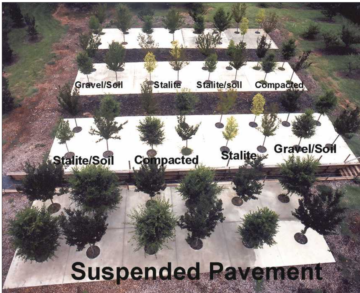
Figure 1. Research plot photographed from above in July 2005, approximately 14 months after plot establishment, labeled to show the different treatments: compacted soil, Stalite, Stalite/soil mixture, gravel/soil mixture, and suspended pavement over noncompacted soil.
