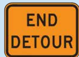
End Detour Sign (M4-8a)
