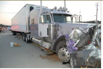
On June 25, 2015, a Peterbilt truck-tractor in combination with a 2005 Great Dane semitrailer was traveling northbound on Interstate 75, near Chattanooga, Tennessee, when it struck the rear of a 2010 Toyota Prius at an estimated speed of 78–82 mph. Traffic had slowed because of road construction and a work zone lane closure. The truck-tractor continued forward and collided with seven additional vehicles. Of the 18 vehicle occupants, 6 died and 4 were injured.
