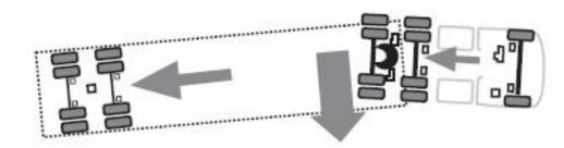
The system automatically reduces engine torque and applies the service brakes (based on the projected rollover risk) to reduce the vehicle speed, thereby reducing the tendency to roll over.
