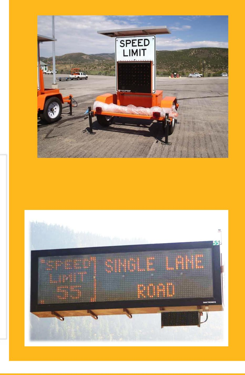
A Utah DOT study shows that the use of Variable Speed Limit signs result in both a statistically significant reduction in speeds through a work zone and a reduction in standard deviation of speeds. The decrease in mean speed can lead to reduced crash severity, while the decrease in speed variance can lead to a reduction in aggressive driving behavior.
